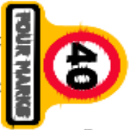
Nearside gateway detail for the 40mph entry point
